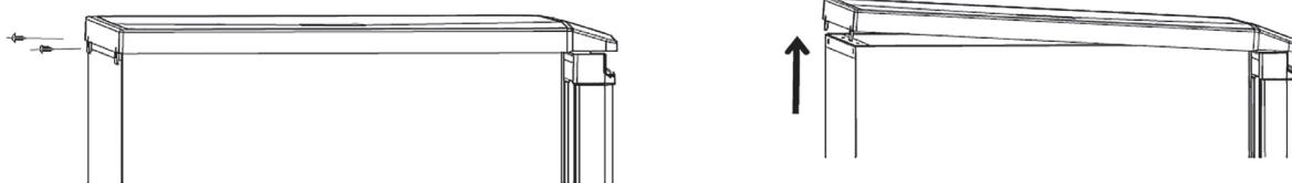
4) Unscrew screws for upper hinge Remove the upper hinge.
